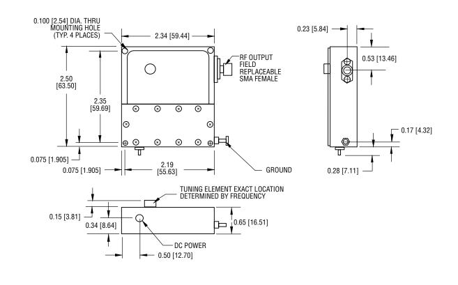
NOTE: DIMENSIONS SHOWN IN BRACKETS [ ] ARE IN MILLIMETERS.
