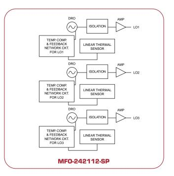
The latest multifunction oscillators, the MFO series subsystem, are three temperature-compensated DROs with frequency tracking to a mathematical algorithm. As shown in the block diagram, the triple oscillator subsystem consists of three DROs at three different frequencies in X- thru K-band that are temperature compensated and track frequency to the following equation:
