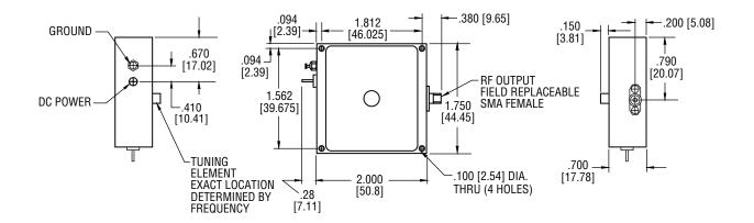
NOTE: DIMENSIONS SHOWN IN BRACKETS [ ] ARE IN MILLIMETERS.
