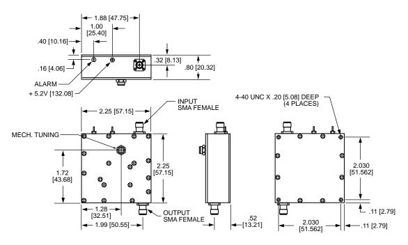
NOTE: DIMENSIONS SHOWN IN BRACKETS [ ] ARE IN MILLIMETERS.
