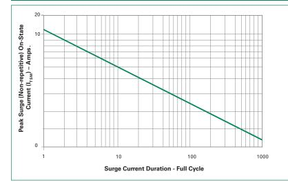
Supply Frequency: 60Hz Sinusoidal Load: Resistive RMS On-State Current [I<sub>T(RMS)</sub>]: Max Rated Value at Specific Case Temperature Notes: 1. Gate control may be lost during and immediately following surge current interval. 2. Overload may not be repeated until junction temperature has returned to steady-state rated value.
