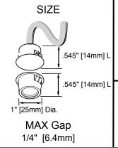
Magnasphere Electrical Specifications Max Current: 0.25A Resistive Max Voltage: 30 VDC Max Power: .25 W Resistive
