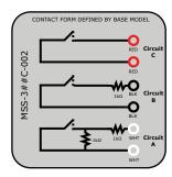
MSS-3##C-002: Series & Parallel 1k resistors on circuit A,
