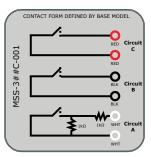
MSS-3##C-001: Series & Parallel 1k resistors on circuit A. One instance shown at right:
