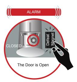
MAGNASPHERE's contact is a spherical magnet and operates in a defined activation zone directed toward the door magnet.
