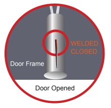
Once contacts have welded closed, they remain in that state though the door is open. They FAIL SECURE.
