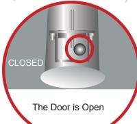
Because the magnet ball contact will not weld, when the door is opened the contact will close and the SYSTEM WILL ALARM.
