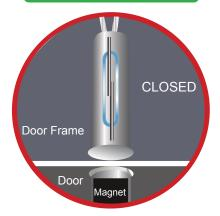
Reed contacts operate on magnetic fields. Most contacts are Closed in the secure position (Closed Loop) when the door is closed and the magnet is near the switch.
