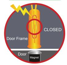
When closed reed contacts are exposed to power surges such as lightning strikes, they are prone to permanent contact welding.
