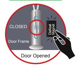
Introducing a defeat magnet OUTSIDE the door will keep the reed contacts closed, allowing an intruder to enter without alerting the security system. They FAIL SECURE.
