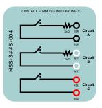
MSS-3##S-004: Series 1k resistor on Circuit A and on Circuit B. One instance shown at right:
