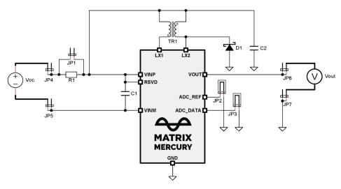
Figure 1: Connection block diagram of MCRY-EVALKIT during quick start
