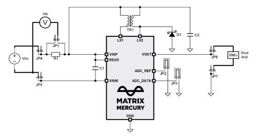
Figure 3: Connection block diagram of MCRY-EVALKIT for detailed measurements
