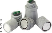
low power 3V - 5.5V operation provides very short to long-range detection and ranging, in a tiny and compact form factor. The I2CXL-MaxSonar-WR will typically detect objects from 0-cm to 765-cm or 1068-cm (select models) (3-cm to 625-cm for the WRC) and provide sonar range information from 20-cm out to 765-cm or 1068-cm (select models) with 1-cm resolution. Objects from 0-cm (3-cm for the WRC) to 20-cm typically range as 20-cm.
