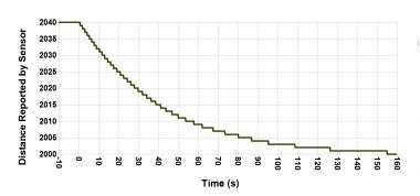
MB7354 responding to a 4 centimeter change. This shows the 7-mm rate limit along with the exponential filter.
