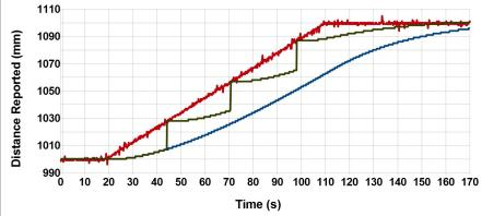
Top (red): MB7364 reporting a target moved from 1 meter to 1.1 meters in a linear fashion. Middle (green): MB7334 responding to the same target, notice the steps when the target moves > 2%.
