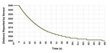
MB7554 responding to a 4 centimeter change. This shows the 7-mm rate limit along with the exponential filter.
