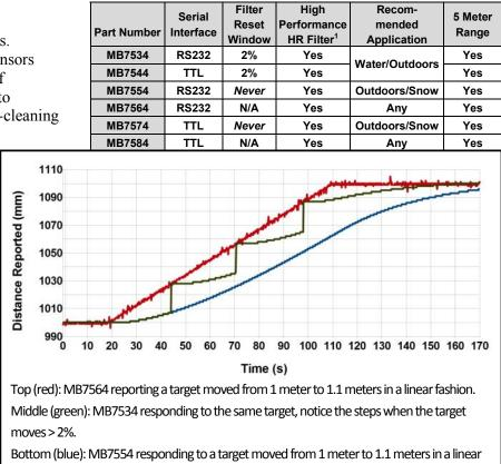
The MB7534 and MB7544 have an additional filter similar to the MB7554 and MB7574 except that the filter will reset to targets that are considered valid outside of a 2% distance to target window. This makes the sensor an ideal balance for accurately monitoring slow or stationary targets that occasionally move rapidly.
