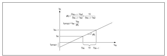
Figure 1. Effective Differential Input Resistance/Offset Current
