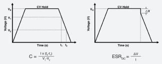
where C is the capacitance (F); I is the absolute value of the discharge current (A);
