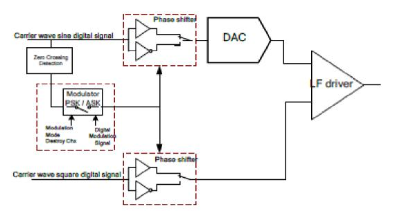
Figure 8: Modulator block diagram
