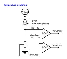
Figure 19: Temperature monitoring: schematics principle
