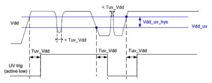
Figure 18: VDD Under voltage: timing diagram
