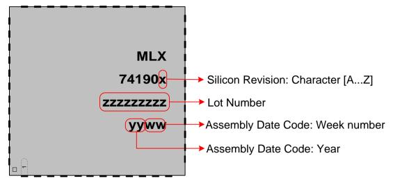
Figure 23: Marking example on IC package TQFP EP 7x7
