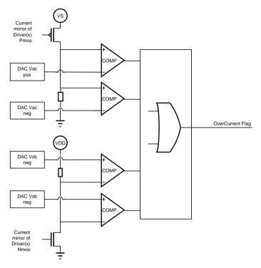
Figure 16: Over Current detection block, schematics principle
