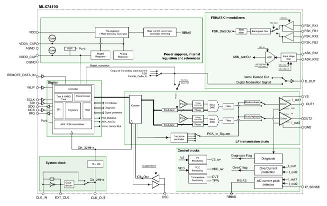
Figure 3: MLX74190 high level block diagram
