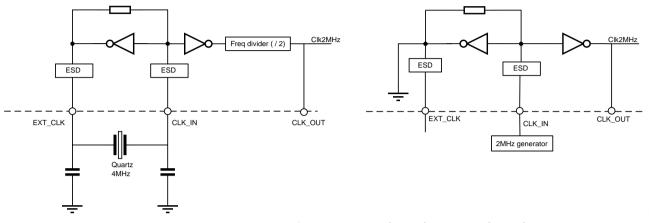
e 6: Dual system clock configuration, MCU (2MHz) or Crystal (4MHz)
