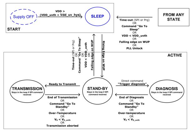
Figure 4: MLX74190 operating modes transition diagram
