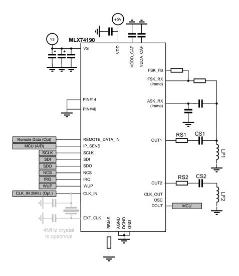
Figure 20: typical application schematic passive start
