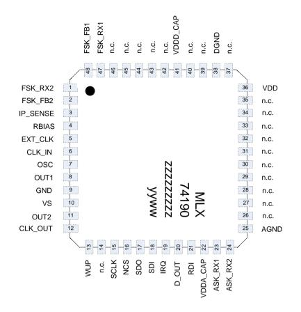
Figure 2: Top view of the package TQFP48
