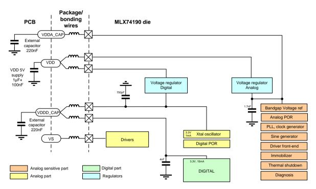
Figure 5: MLX74190 Power supplies, internal regulators and references
