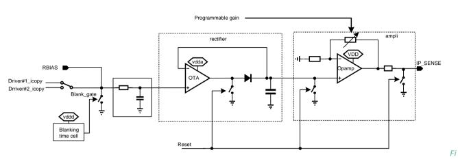
gure 15: Current measurement, schematics principle
