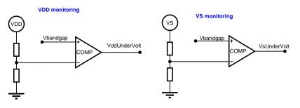
Figure 17: Under voltage detections, schematics principle
