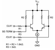
Figure 2a. CLK1 Differential Input Structure
