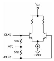
Figure 2b. CLK0 Differential Input Structure
