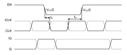
Set-Up and Hold Time EN-to-Differential IN
