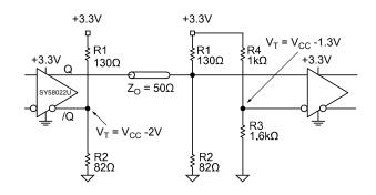
Figure 6. Terminating Unused I/O
