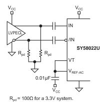
$R_{\rm pd}^{\rm pd}$  = 50 $\Omega$  for a 2.5V system.
