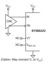
Figure 3d. AC-Coupled CML Input Interface
