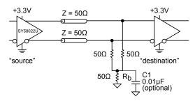
Figure 5. Three-Resistor "Y-Termination"
