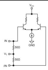
Figure 2. Simplified Differential Input Buffer
