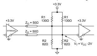
Figure 4. Parallel Termination-Thevenin Equivalent
