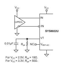
Figure 3a. DC-Coupled LVPECL Input Interface
