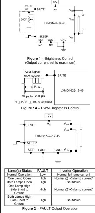
Under some conditions the second lamp will also shutdown, this is especially true if the inverter draws an arc going open or when shorted
