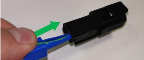
5. Remove the tool from the contact. Pull back lightly on the wire to ensure that the contact is secure in the cavity.
