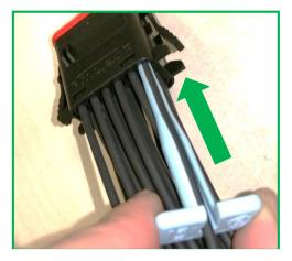
STEP 1: With rear of connector pointed towards you, snap the removal tool (p/n: 63813-1900\*) over the cable of the contact to be removed
