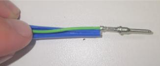
2. Slide the contact wire barrel into the insertion (blue) end of the tool tip until the tip butts against the shoulder of the contact.
