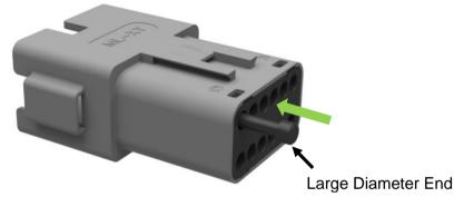
Step 3: Apply pressure until sealing plug is forced to stop by contact with the back cover. Visually inspect the sealing plug large diameter end to confirm it is flush with cavity opening. If multiple sealing plugs are used close together, the large ends may not sit flush due to tight spacing. Maximum allowable distance from top of sealing plug to grommet surface is 5.00mm.
