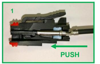
To ensure secure terminal insertion: Follow the Push, Click, Pull Method of terminal insertion
