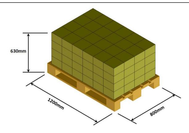
Figure 5: Pallet Layout Diagram
