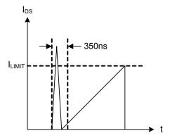
Figure 5—Leading-edge blanking
