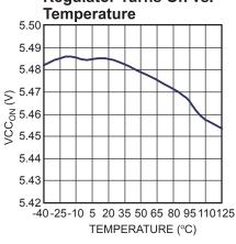
VCC Decreasing Level at which the Protection Phase Ends vs.
