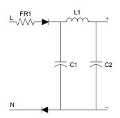
Figure 8—Half-wave rectifier
