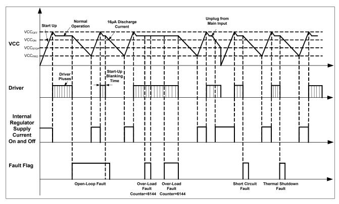
Figure 11—Signal evolution in the presence of a fault
