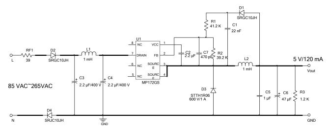
Figure 9—Typical application at 5 V, 120 mA
