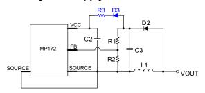
Figure 7—Auxiliary Vcc supply circuit
