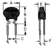
Lead Size : 24 AWG Ø0.51mm Diameter
