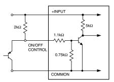
Figure 2a. Inverting On/Off Control Pin Signal and Power-Up Sequencing
