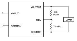
Note: Install either a fixed trim-up resistor or a fixed trim-down resistor depending upon desired output voltage.
