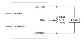
Figure 3. Trim Connections Using a Trimpot
