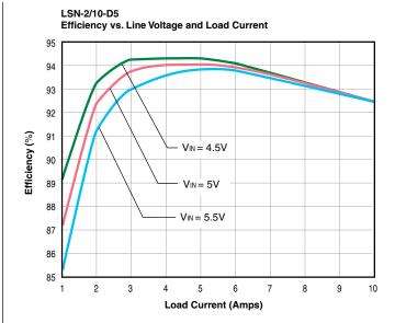
LSN-2.5/10-D5 Efficiency vs. Line Voltage and Load Current
