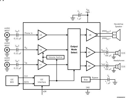
FIGURE 1. Typical Audio Amplifier Application Circuit
