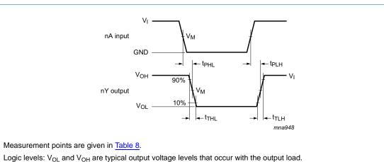
Fig 6. Input (nA) to output (nY) propagation delays
