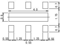
\* : Dummy pattern should be floating or soldering to PCB
