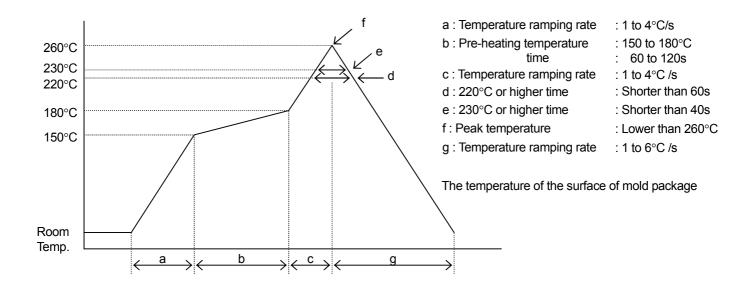
(NOTE1) Using reflow furnace with short wave infrared radiation heater such as halogen lamp Regarding temperature profile, please refer to those fo reflow furnace.
