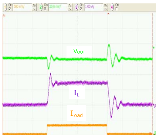
Figure 15. MODE=1, 100 mA to 1.5 A to 100 mA, 5 \mu\text{s}/\text{div} .
