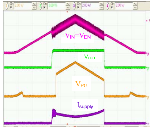
Figure 20. Soft-Start, EN Pin Tied to VCC R_{LOAD}=400\text{ m}\Omega , C_{OUT}=100\text{ }\mu\text{F} , 1\text{ ms/div} .
