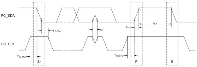
Figure 2. I<sup>2</sup>C Mode Timing
