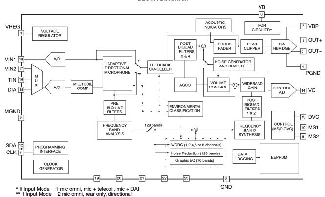
Figure 1. Hybrid Block Diagram
