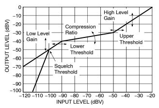
Figure 6. Independent Channel I/O Curve Flexibility
