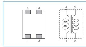
• The pin numbers shown here are for reference purposes only. Confirm the actual pin number arrangement with the exchanged specification documents.
