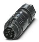
Circular connectors (cable-side), Range of articles: PRC, Coupler connector, type: Can only be released with a tool, housing material: PPE, color: black, number of positions: 3, min. conductor cross section: 1.5 mm², max. conductor cross section: 6 mm², nom. voltage: 690 V AC, rated current: 35 A, Connection method: Screw connection, Type of contact: Socket, min. cable diameter: 8 mm, max. cable diameter: 12 mm. Variant for release with a tool
