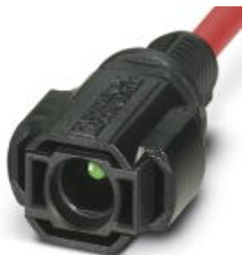
Photovoltaic connector, Photovoltaic connector, housing material: PPE, color: black, number of positions: 1, min. conductor cross section: 6 mm 2 , Connection method: Crimp, Type of contact: Pin, cable length: 130
