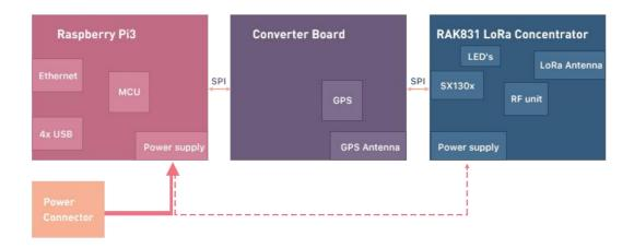
Figure 5.1: Hardware structure
