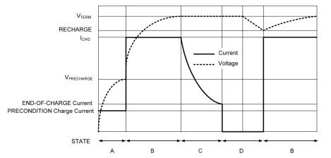
A: PRECONDITION State B: FAST-CHARGE State C: TOP-OFF State D: END-OF-CHARGE State
