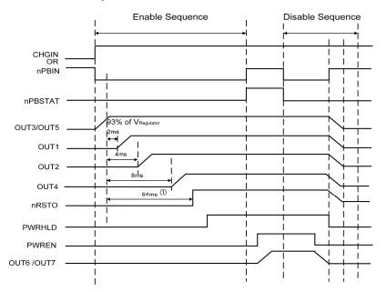
D: Typical value shown, actual delay time may vary from (T-1ms) x 88% to T x 112%, where T is the typical delay time setting.
