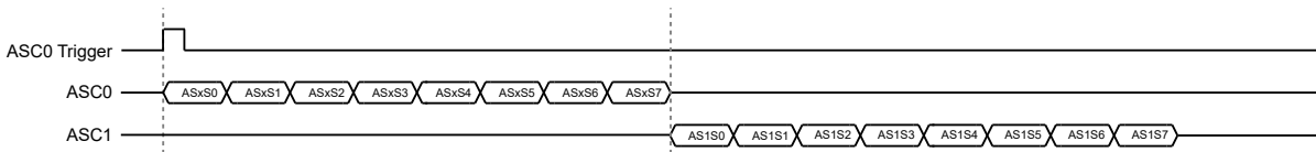
Figure 17-5. ASCx, ADCCTL.ADCMODE = 011b, 110b
