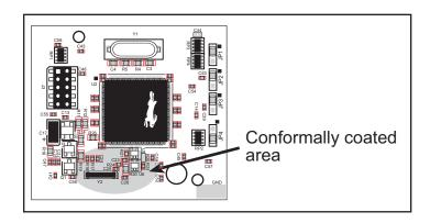
Figure A-5. RCM3100 Areas Receiving Conformal Coating
