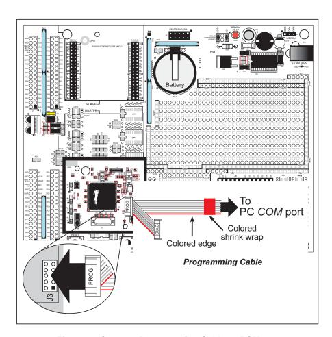
Figure 2. Connect Programming Cable to RCM3100
