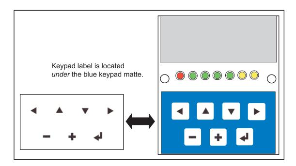
Figure C-5. Removing and Inserting Keypad Label
