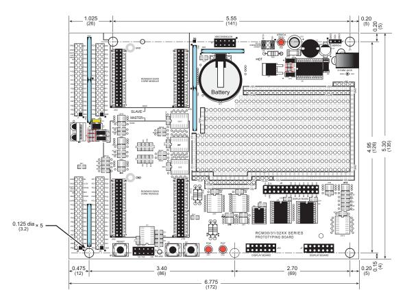
Figure B-2. RCM30/31/32XX Prototyping Board Dimensions
