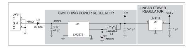
Figure B-3. Prototyping Board Power Supply
