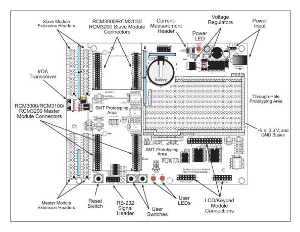
Figure B-1. RCM30/31/32XX Prototyping Board
