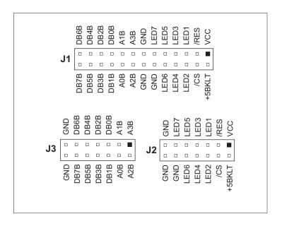
Figure C-6. LCD/Keypad Module Pinouts
