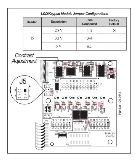
Figure C-3. LCD/Keypad Module Voltage Settings
