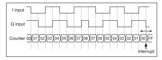
Figure E-2. Operation of Quadrature Decoder Counter
