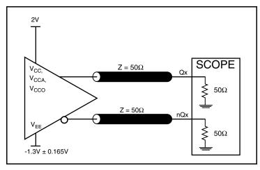
3.3V LVPECL Output Load AC Test Circuit
