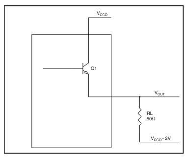
Figure 5. LVPECL Driver Circuit and Termination
