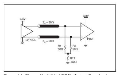
Figure 3A. Figure 4A. 3.3V LVPECL Output Termination
