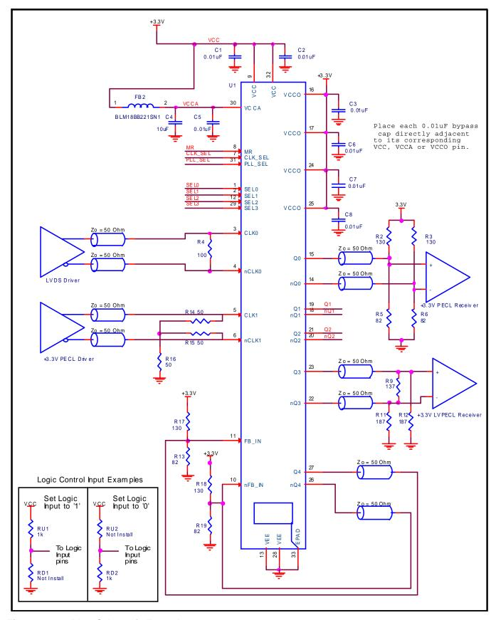
Figure 4. 8735BI-01 Schematic Example
