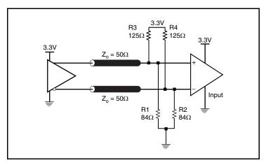
Figure 3B. Figure 4B. 3.3V LVPECL Output Termination
