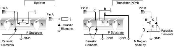
Figure 7. Example of monolithic IC structure
