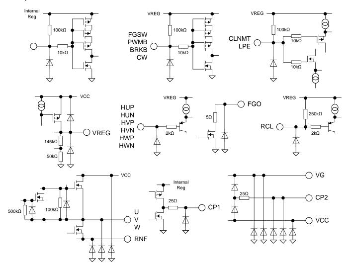
Figure 6. I/O Equivalence Circuits
