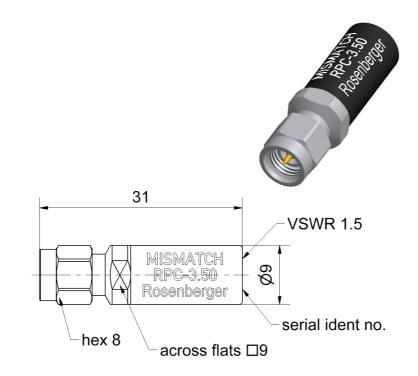
All dimensions are in mm; tolerances according to ISO 2768 m-H
