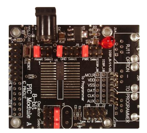
Schmartboard Development Board A for the 8 Bit PIC® Microcontroller
