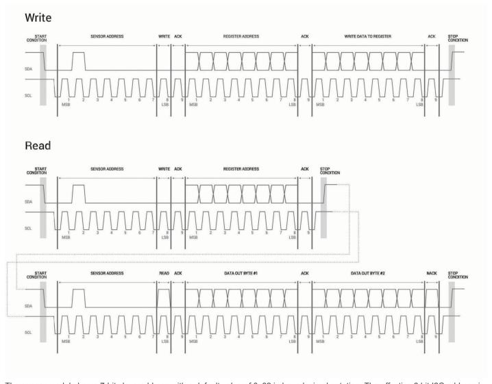
The sensor module has a 7-bit slave address with a default value of 0x62 in hexadecimal notation. The effective 8 bit I2C address is 0xC4 write, 0xC5 read. The device will not respond to a general call.
