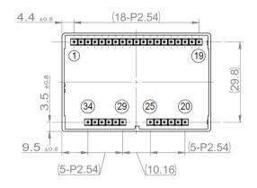
Note :1.The dimensional tolerance without directions is  $\pm$  0.5mm.
