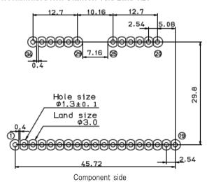
XThe round pulling out figure is a pin numbering.
