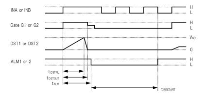
Timing chart of short circuit protection function
