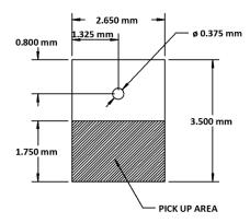
Figure 17. Recommended Vacuum Pick-up Area
