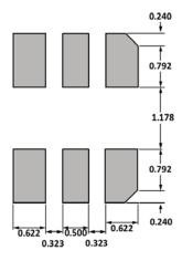
Figure 94. Recommended PCB Land Pattern Layout
