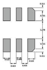
Figure 105. Suggested Solder Paste Stencil Pattern Layout
