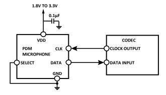
Figure 71. Mono PDM Microphone (Right Channel) Connection to Codec
