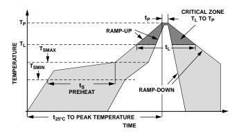
Figure 2. Recommended Soldering Profile Limits
