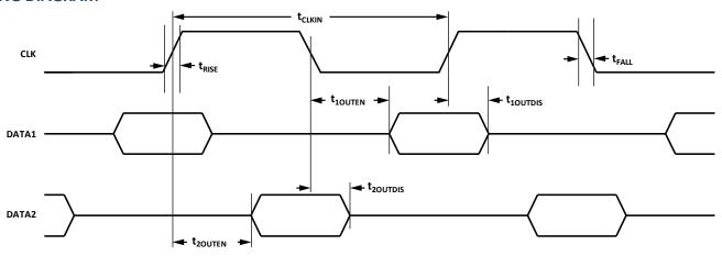
Figure 1. Pulse Density Modulated Output Timing
