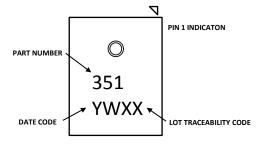
Figure 128. Package Marking Specification (Top View)
