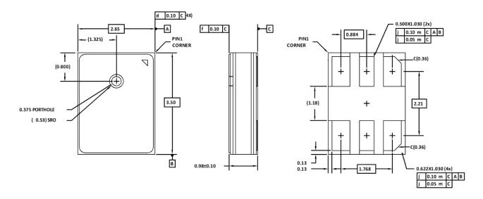
Figure 116. 6-Terminal Chip Array Small Outline No-Lead Cavity 3.50 mm × 2.65 mm × 0.98 mm Body
