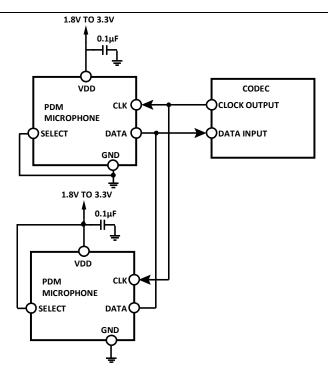
Figure 82. Stereo PDM Microphone Connection to Codec
