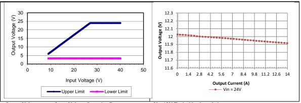
Output Voltage versus Input Voltage Operating Range
