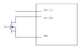
On/Off Circuit for positive or negative logic
