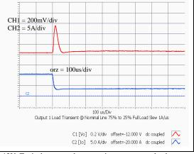
Vo=12V Typical output voltage transient response to load step from 75% to 25% of full load with output current slew rate of 1A/uS. (Cext = 3x47uF ceramic capacitor)
