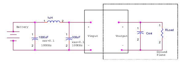
The input reflected ripple is measured with a current probe and oscilloscope. The ripple current is the current through the 1uH inductor.
