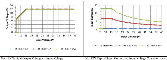
Vo=12V Typical Output Voltage vs. Input Voltage Characteristics
