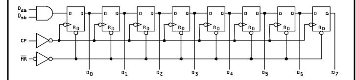
FIGURE 3. Logic diagram.
