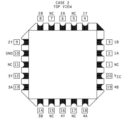
FIGURE 1. Terminal connections and logic diagram.
