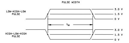
FIGURE 4. Switching waveforms and test circuit.
