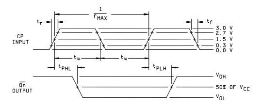
FIGURE 4. Switching waveforms and test circuit.
