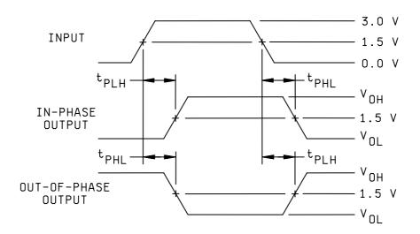
FIGURE 3. Test circuit and switching waveforms.
