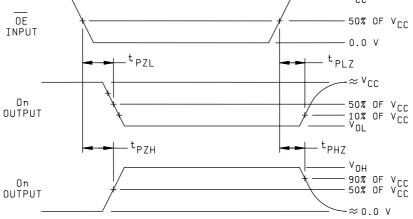
FIGURE 4. Switching waveforms and test circuit.
