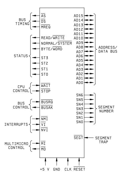
FIGURE 3. Logic functions.
