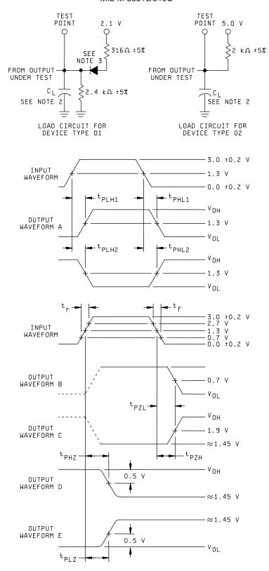
FIGURE 4. Switching test circuit and waveforms for device types 01 and 02 - Continued.
