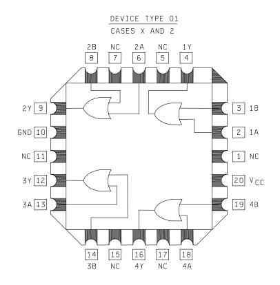
FIGURE 1. Terminal connections and truth table.
