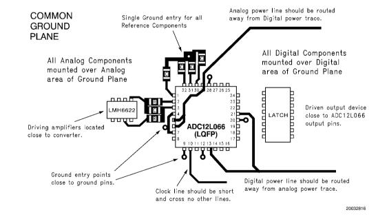
FIGURE 7. Example of a Suitable Layout
